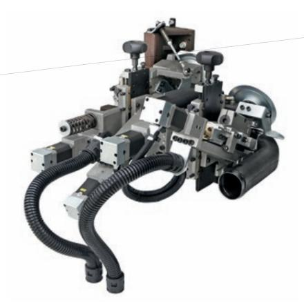
The Edge-scraper eliminates the imperfections resulting from previous machining operations on the top and bottom of the edge.
