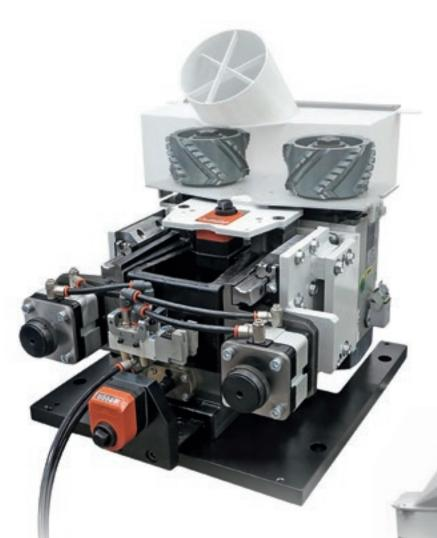
The RT20 2-motor Pre-milling Unit with automatic intervention guarantees a perfect base for gluing.
